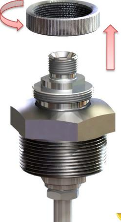
!!CAUTION - Sensor core & Sensor Body are sprung loaded!!
