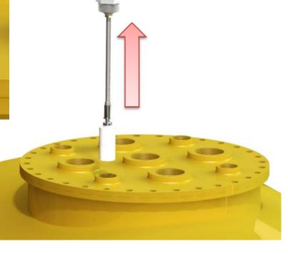
N.B. ONCE REMOVED FROM THE TANK LID, CONTINUE WORK ON THE FLOAT, IN A SAFE AREA TO AVOID UNNECESSARY POTENTIAL SPARKS!
