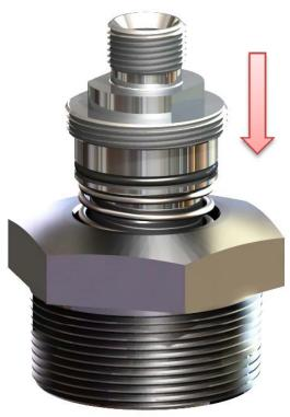
4. Compress the upper portion in the valve body and screw the core together which will engage the upper portion (locking the valve together).
