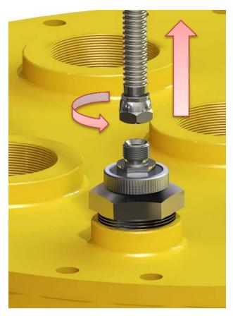
2. Remove flexi hose from float body and fit the red cap supplied to protect threads and prevent ingress of dirt.
