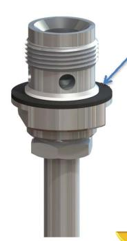
3. Replace Sensor Valve Seal (ensure no grease from "O"-ring comes into contact with the valve seal).
