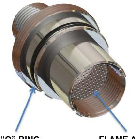
Replace "O"-ring (using "O"-ring grease) and install the flame arrester inside the upper portion of the sensor body.
