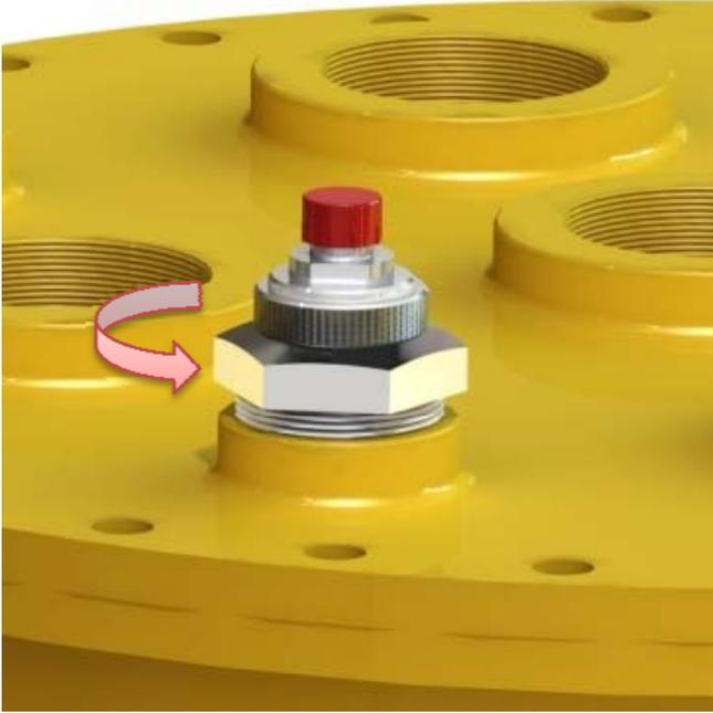
3. Using a large non-spark adjustable spanner (2.5 inch), unscrew the float and remove. Take care not to damage the float tube or foam float assembly.
