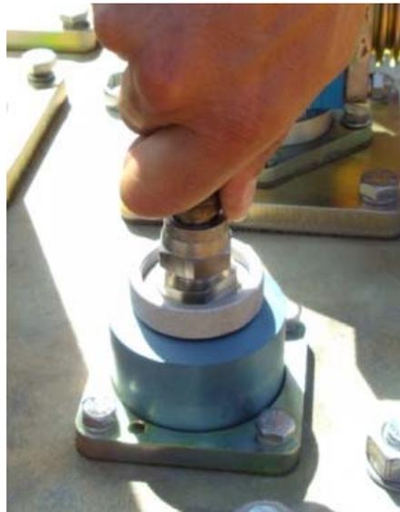
Whilst holding the top down a mild 'thump' and fill hose reaction should be noticed indicating that the shut off valve has closed.
