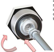
Insert the drop tube with olive assembly into the cartridge as shown. Tighten the clamping nut over the olive to hold the cartridge in situ, ensuring that the olive is properly compressed.
