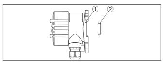
Fig. 4: VEGADIS 82 with plastic housing for carrier rail mounting
