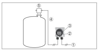
Fig. 2: Connection of VEGADIS 82 to the sensor
