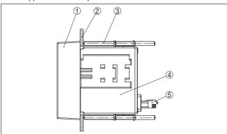
Fig. 7: VEGADIS 82 for panel mounting
