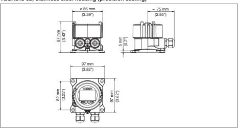
Fig. 23: VEGADIS 82, with stainless steel housing (precision casting)
