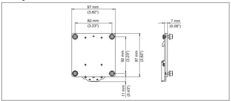
Fig. 24: Adapter plate for carrier rail mounting of VEGADIS 82
