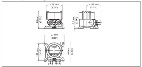
Fig. 20: VEGADIS 82 with plastic housing
