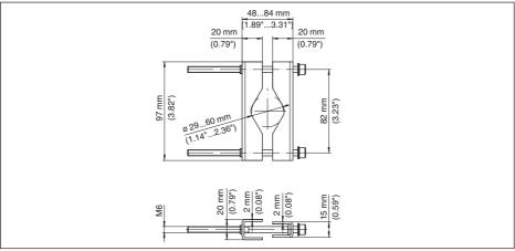
Fig. 25: Brackets for tube mounting of VEGADIS 82
