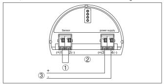
Fig. 12: Bridge on terminals 1 and 2 on the VEGADIS 82
