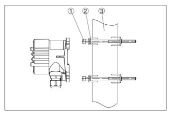
Fig. 6: VEGADIS 82 for tube mounting
