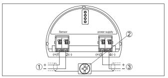
Fig. 9: Wiring plan VEGADIS 82 for 4 ... 20 mA sensors
