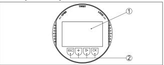
Fig. 17: Display and adjustment elements
