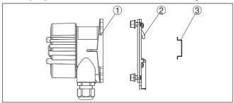
Fig. 5: VEGADIS 82 with aluminium and stainless steel housing for carrier rail mounting
