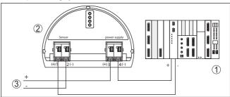
Fig. 14: Connection of VEGADIS 82 as external display to four-wire sensors with active 4 ... 20 mA output with additional processing system/PLC
