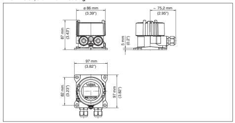
Fig. 22: VEGADIS 82 with Aluminium housing
