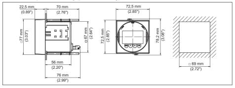
Fig. 21: VEGADIS 82 with plastic housing for panel mounting
