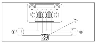
Fig. 10: Wiring plan VEGADIS 82 for 4 ... 20 mA sensors - panel mounting
