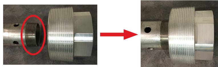
4. Apply a UL-approved, stay-soft (non-hardening), fuel-resistant pipe sealant to the threads at the bottom of the mini-Jet, and then thread it into the top of the drop tube adapter.
