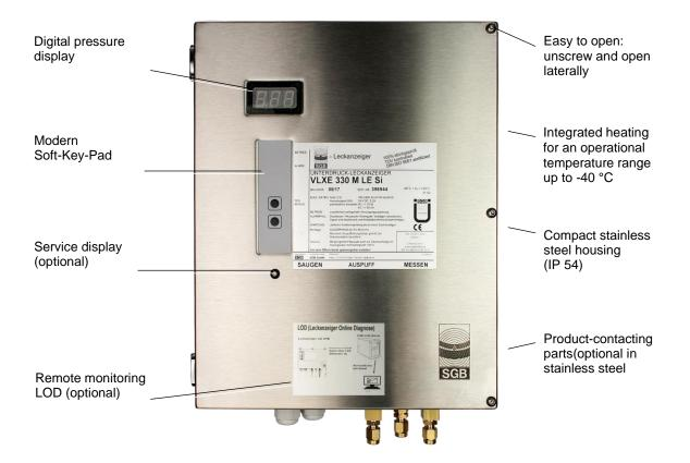
A leak prevention system which realizes the highest European environmental protection level of EN 13160, class I
