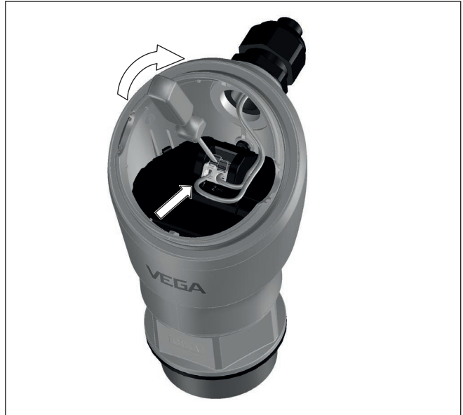
Fig. 19: Connection steps 5 and 6
