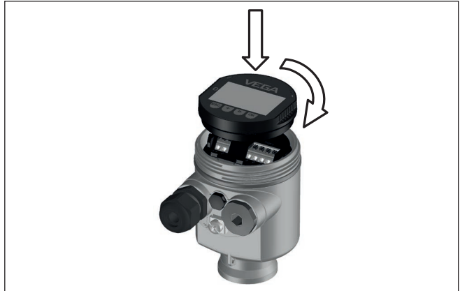
Fig. 3: Installing the display and adjustment module in the electronics compartment of the single chamber housing
