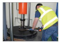
The covers are load tested in accordance with the new EN124 2015 directive to exceed a 400kn (40t) load rating far in excess of any load it will see in normal traffic conditions.
